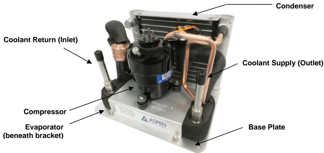
Figure 1: LCM (FP00039) Assembly (drive board and cable not shown)
