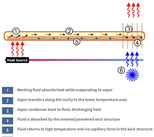
Natural or forced convection air flow dissipates excess heat to ambient
